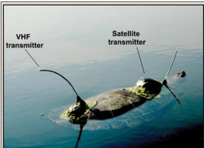
FIG. 4. Satellite and VHF Transmitters glued on the carapace of the turtle (*Podocnemis expansa*) with Turbolit. The paste is molded onto the turtle shell, followed by pressing the transmitter into the paste and folding it over the transmitter to make a secure bond. In this picture the turtle has just been released.
