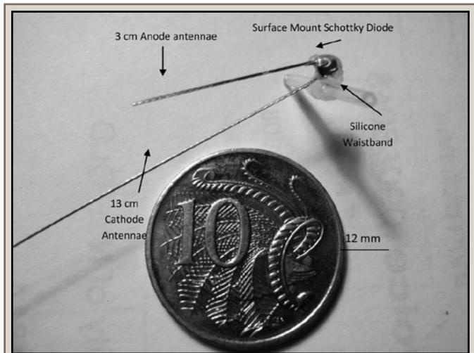
FIG. 1. A dipole harmonic tracking device with an Australian 10-cent coin (23 mm diameter) for scale.
