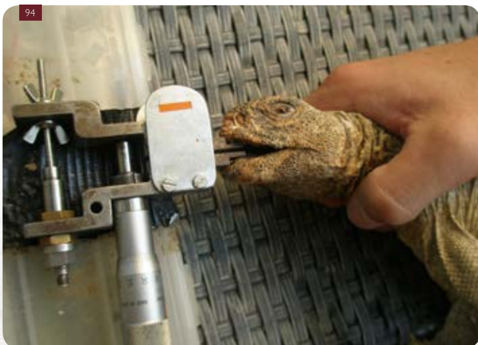
Bite forces were measured in Qatari Dhubs and we discovered that males and females with similar body size also have similar bite forces. The maximal bite forces recorded in the Dhub is of 141 Newtons (Herrel et al. 2014)
