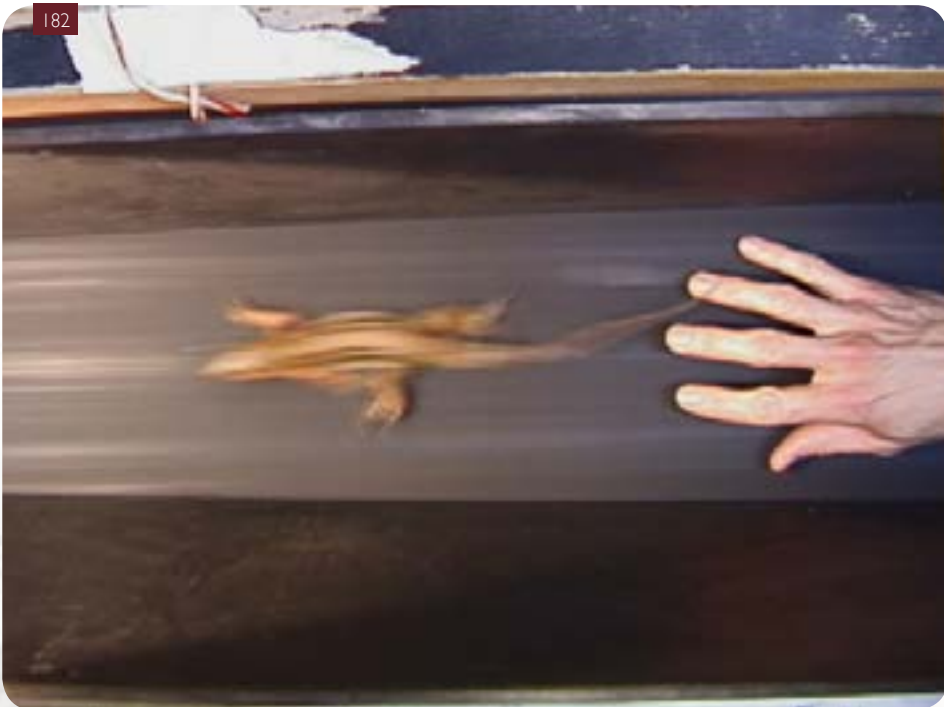
High-speed treadmill connected to a computer that can rapidly reach 45 km/h. This is used to measure maximal running speeds of lizards that are chased with the hand simulating a predator
