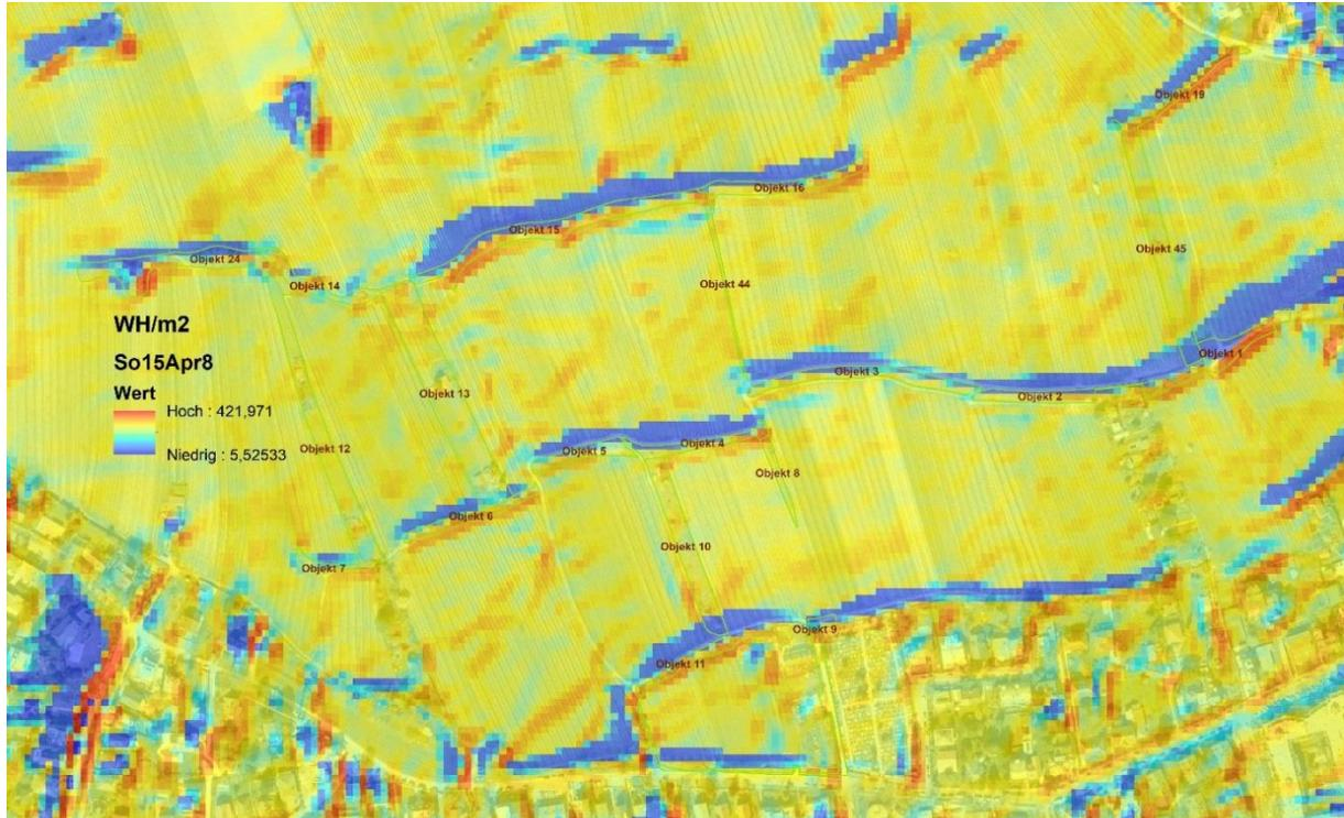
Figure 15: Solar insolation on April 15th 08:00 morning, blue patches show areas with low insolation around 5 WH/sqm, orange and red parts show high insolation up to 422 WH/ sqm. Created with ArcGIS
