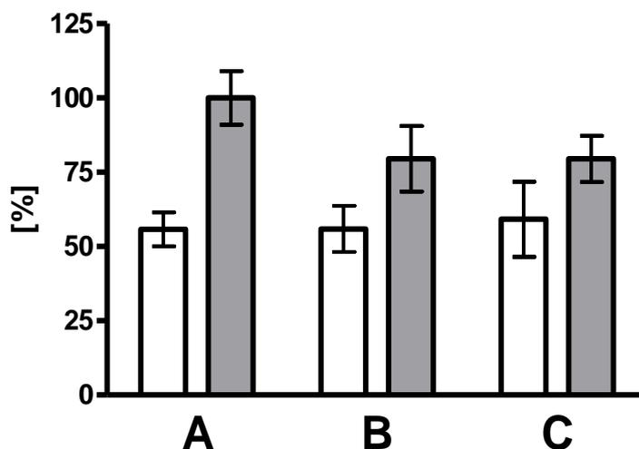
**Figure 1:** Evaluation of extraction solvent and dSPE sorbent. Sum of the peak areas of all 9 pesticides ( $1.50 \text{ mg kg}^{-1}$ ) expressed in %. **White** acetone/nitrile, **grey** ethyl acetate; **A** 75 mg PSA:MgSO<sub>4</sub>, (1:4); **B** 75 mg PSA:C18EC:MgSO<sub>4</sub> (1:1:4), **C** 75 mg Agilent QuEChERS dSPE EMR-Lipid®; error bars show the standard error of the mean (SEM) (n = 6).
