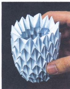
A variable-diameter origami wheel in prolate spheroid configuration
